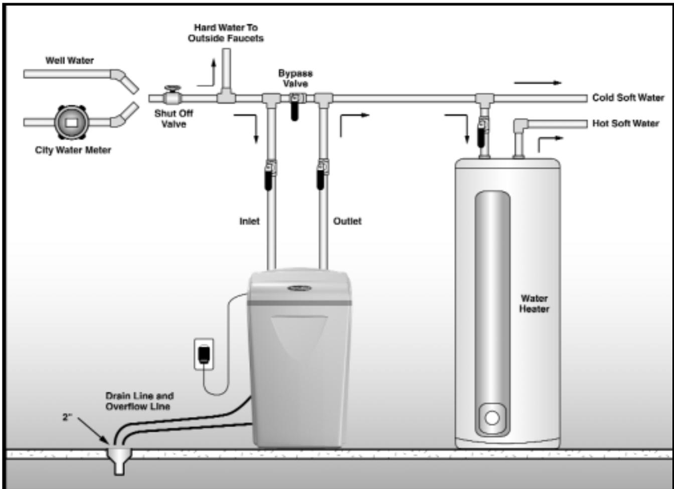
Use this diagram as a location and installation guide for your **WaterBoss®700**, **WaterBoss®900**, and **WaterBoss®550**, water conditioners. This diagram applies to all types of installations (i.e. basement, slab, crawl space, outside).
