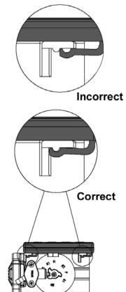
Figure 8: Controller Tab Lock Detail
