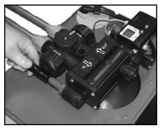
Figure 5: Connect Drain Line
