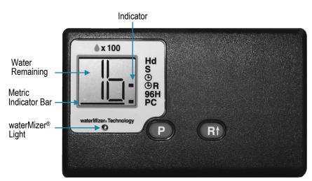
Figure 7: Two-Button Controller
