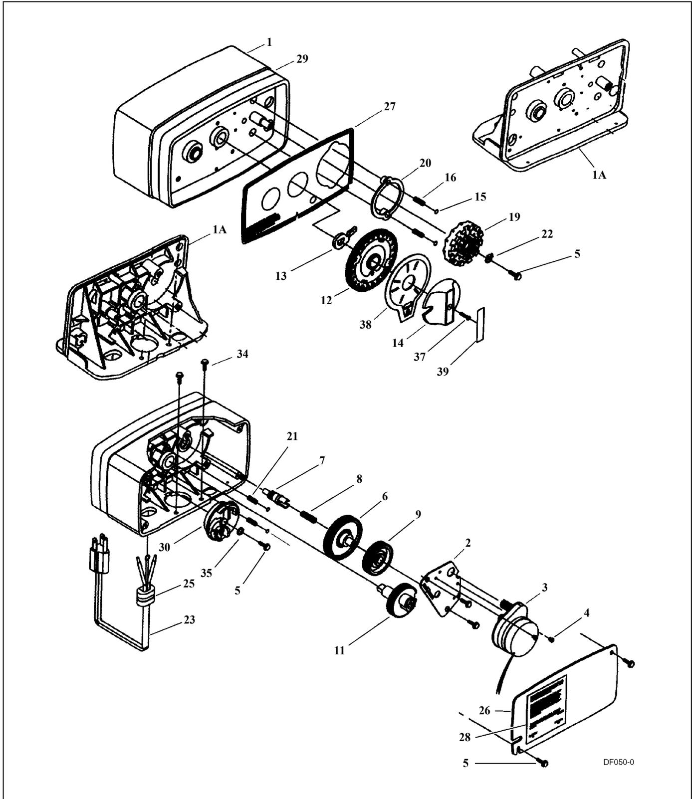
Figure 12: Model 5600 Control Valve Drive Assembly
